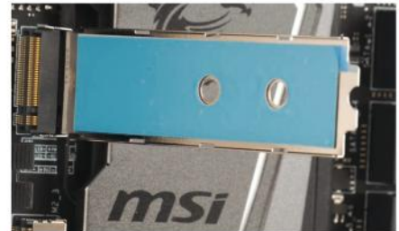
There’s a cooling pad behind the M.2 Shield, giving M.2 SSDs better cooling for longer lifespans
