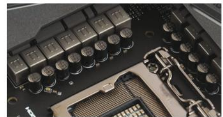
The Gaming M7 has more power phases to provide more power and stability for overclocking
