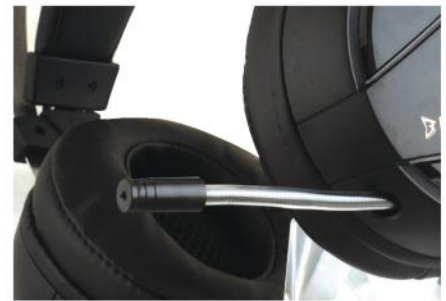
You can slide the microphone in when not in use, and the earcups pulse and vibrate to sounds created by the speakers
