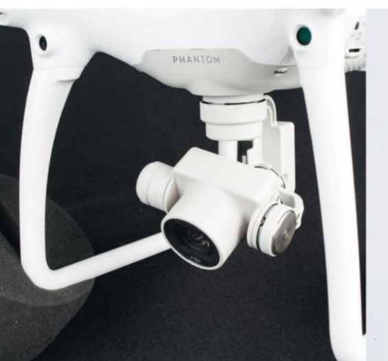
The motorised camera suspension of the DJI Phantom 4 counterbalances all of the drone's movements and vibrations
