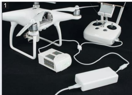
The remote control of the DJI Phantom 4 1 accommodates a smartphone. An app displays live images and facilitates adjustments. For re-charging, the battery and remote control are attached to the DJI mains adapter 2
