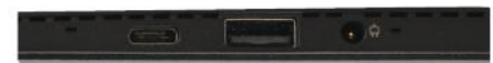
The Miix 510 sports both a USB 3.0 Type A and USB 3.1 Type C port
