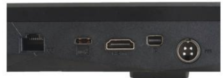
USB Type-C, LAN, HDMI and mini DisplayPort, there's a lot of connectivity options
