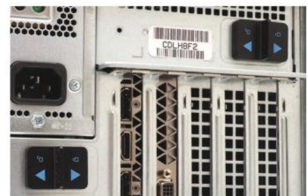
These two latches at the back lock the side panel and PSU compartment in place
